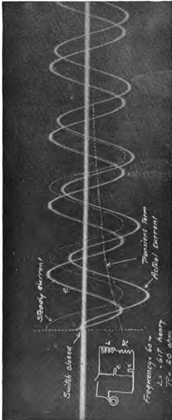
FIG. 42.—The ordinary form of current occurring when switching an inductive circuit to an a.c. supply line; analysis of the actual current is shown by the dotted curves.
